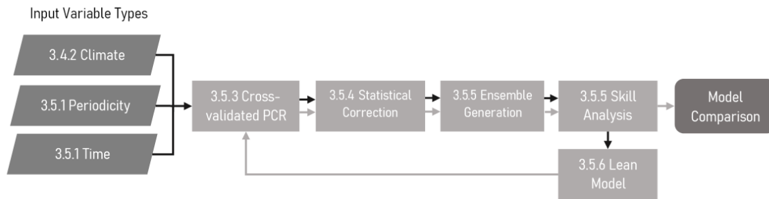
Figure 2. Systematic framework visualization: numbers correspond to section and subsection; black arrows represent the initial model development process, and grey arrows represent how the lean model is developed by reusing the initial process
